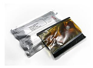
Specially designed for taped resin injection cablejoints up to 10kV. The resin contains polyether polyols, estherpolyols, and fire retardant additives. The hardner is a high quality MDI type. Filofill P2600 does not contain halogens or plasticizers. Filofill P2600 has good anti-corrosion properties and provides good adhesion to metals, ceramics, many different plastics and can be used on all plastic and paper isolated cable types.
